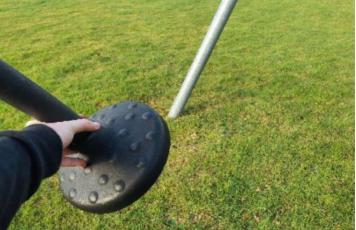
**Finding:** The seat is less than 2.0 metres from the post when extended at 45 degrees at the end of the area of travel minimum distance is maintained and does not meet the requirements of BS EN 1176 Part 4
