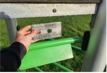
Finding: The item fails to meet the requirements of BS EN Action: Monitor - No action given the risk assessment 1176 Part 1 4.2.7.2 for head and neck entrapment in the frame
