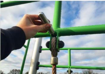
**Finding:** There is/are finger entrapment/s in the frame and the item fails to meet the requirements of BS EN 1176 Part 1
