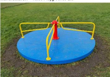
Finding: The distance between the underside of the roundabout platform and the playing surface is less than 60mm and contravenes the requirements of BS EN 1176 Part 5 which requires that the distance be maintained between 60mm-110mm for the entire circumference of the roundabout
